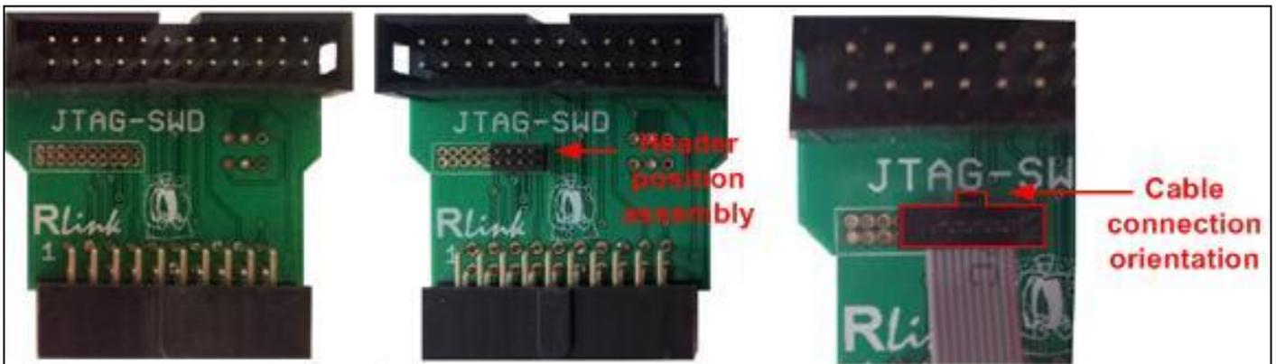
Figure 16: JTAG-SWD - header assembly and connection
