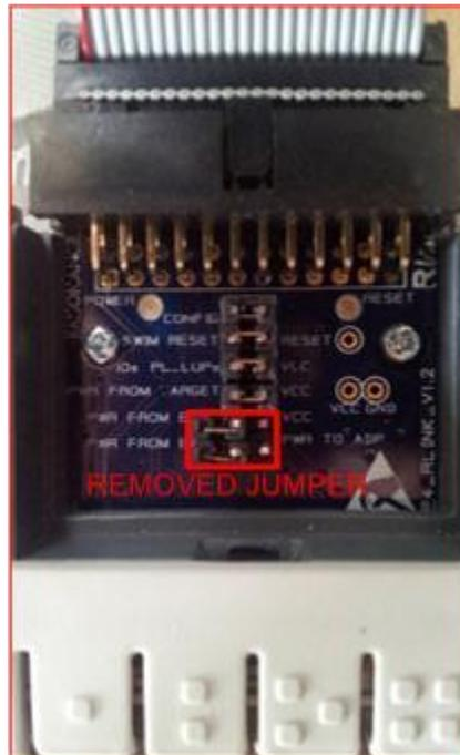
Figure 19: Open4-RLink-ADP Jumper configuration
