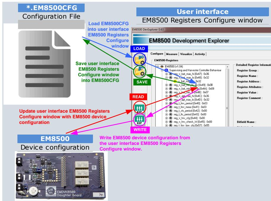
Figure 10-4 EM8500 DevExplorer configuration flow description
