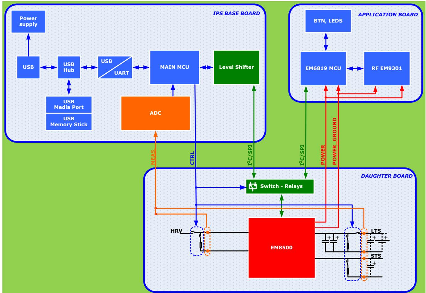
Figure 5-1 EMDVK8500 System Architecture
