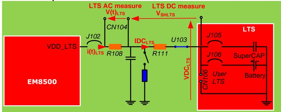
Figure 8-6: LTS measurements
