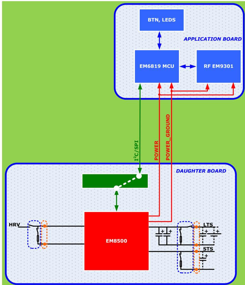
Figure 5-4 EMDVK8500 Stand-alone Mode with default application board
