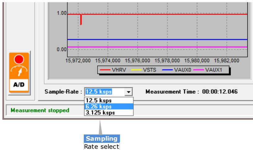
Figure 10-8 EM8500 DevExplorer visualize sampling rate selector
