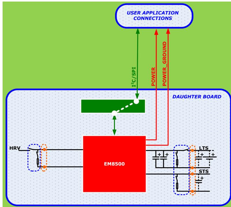
Figure 5-5 EMDVK8500 Stand-alone Mode with user application connections
