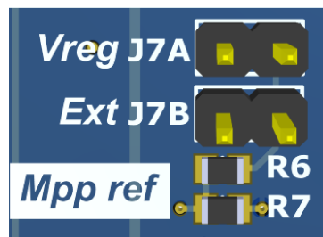
Figure 4-9: EMEVB8504 VMPP configuration schematic configuration area
