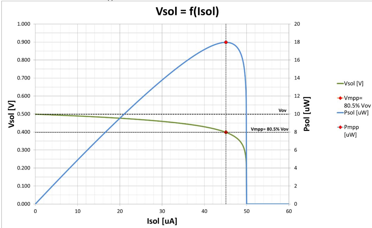
Figure 2:  $V=f(I)$  Curve of a Solar Cell
