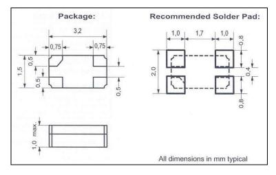
The termination is with Au flashed pads for SMD mounting.
