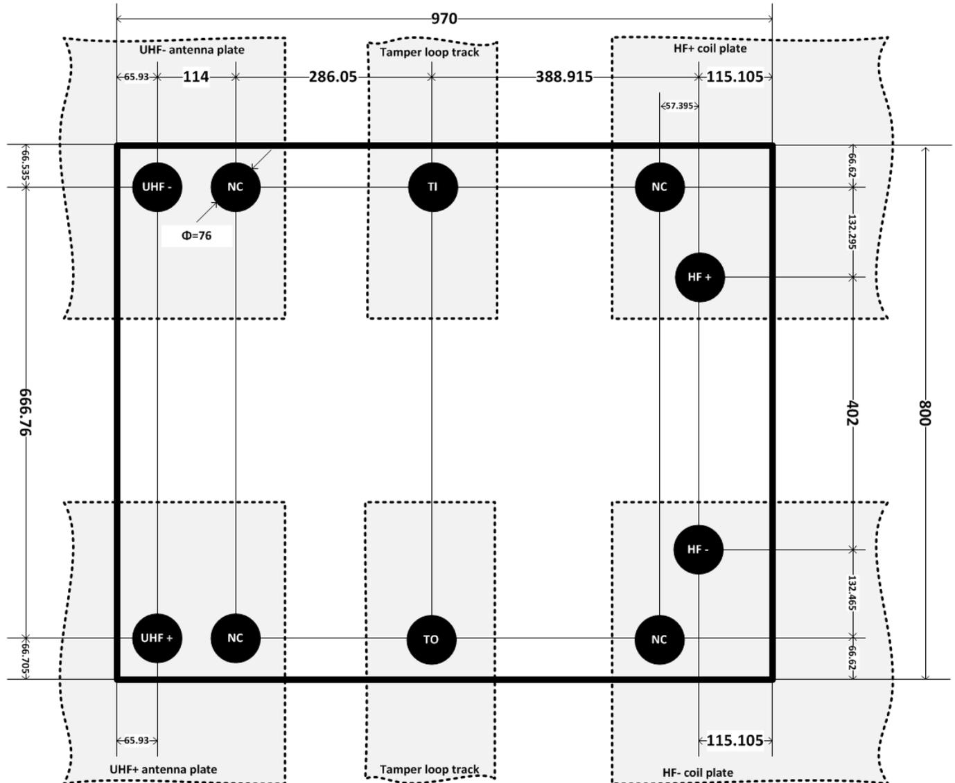
The chip size is calculated including the scribe line. UHF antenna plates and HF coil plates are added here only to illustrate inlay assembly option.
