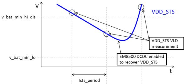
Figure 1: VDD\_STS Measurement Toward v\_bat\_min\_hi\_dis
