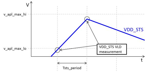
Figure 3: VDD\_STS Measurement Toward v\_apl\_max\_lo
